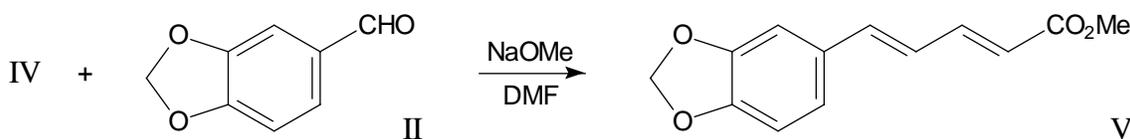
Finally, piperine is synthesized in a trans-amination reaction between **V** and piperidine. This reaction should also not isomerize either of the double bonds.
