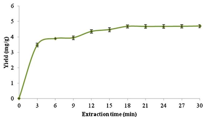
**Fig. 3.** Effect of time on extraction yield of Piperine from *Piper longum* using UAE (ethanol as solvent, solid/solvent ratio of 1:10, extracting time of 30 min, temperature of 40 °C, ultrasonic power of 175 W, frequency of 25 kHz).
