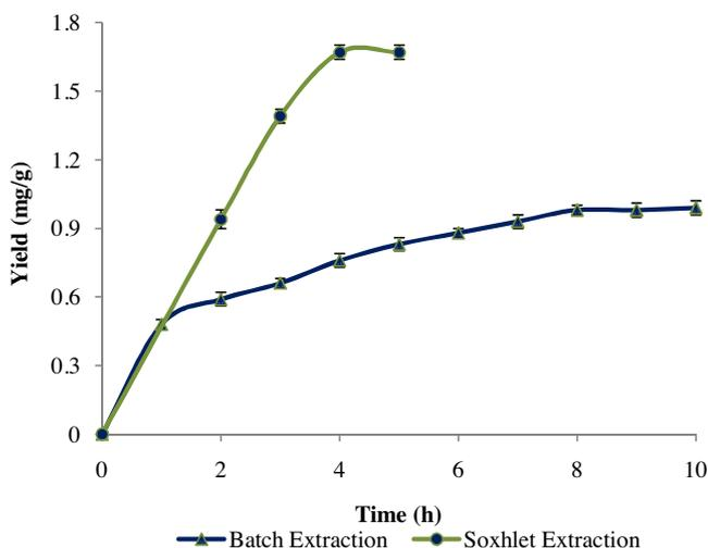
Fig. 9. Extraction yield of Piperine from *Piper longum* with respect to time using traditional methods.
