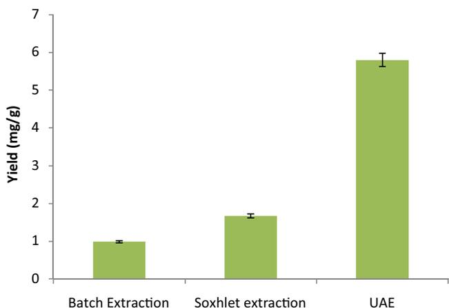
Fig. 10. Comparison of extraction methods with respect to yield of piperine.
