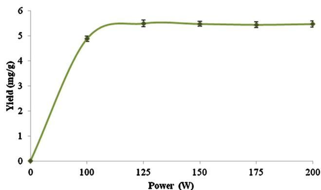
Fig. 7. Effect of ultrasonic power on extraction yield of piperine from *Piper longum* (ethanol as solvent, extracting time of 18 min, solid/solvent ratio of 1:10, temperature of 40 °C, frequency of 25 kHz).
