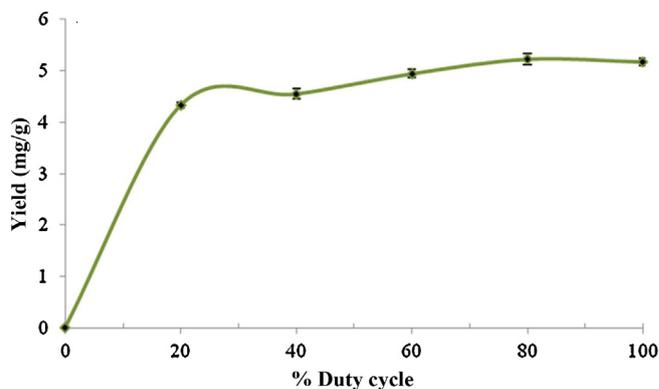
**Fig. 5.** Effect of duty cycle on extraction yield of piperine from *Piper longum* (ethanol as solvent, extracting time of 18 min, solid/solvent ratio of 1:10, temperature of 40 °C, ultrasonic power of 175 W, frequency of 25 kHz).
