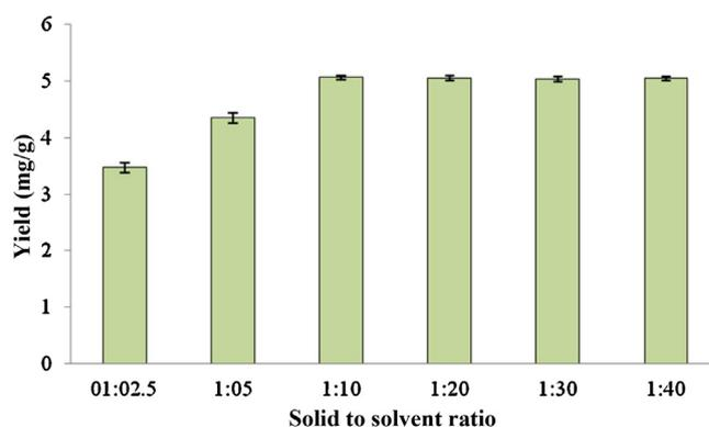
**Fig. 4.** Effect of solid to solvent ratio on extraction yield of piperine from *Piper longum* (ethanol as solvent, extracting time of 18 min, temperature of 40 °C, ultrasonic power of 175 W, frequency of 25 kHz).
