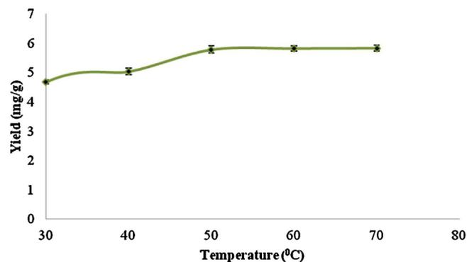
Fig. 8. Effect of temperature on extraction yield of piperine from *Piper longum* (ethanol as solvent, extracting time of 18 min, solid/solvent ratio of 1:10, frequency of 25 kHz, ultrasonic power of 125 W).
