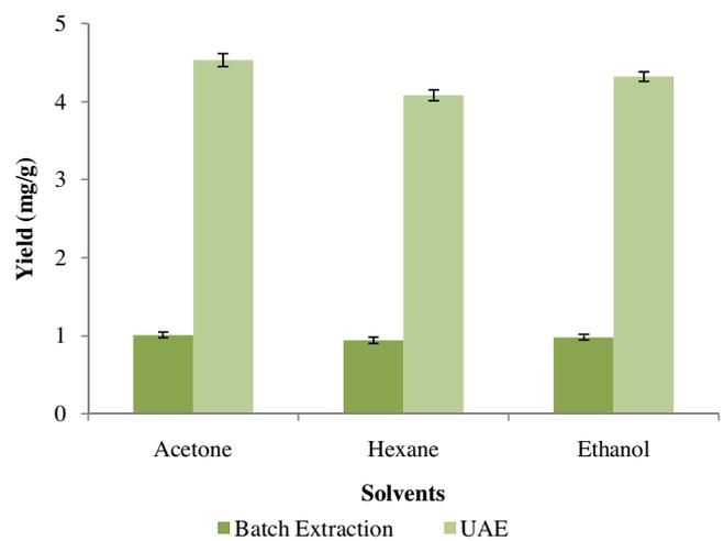
**Fig. 2.** Effect of different solvent on extraction yield of Piperine from *Piper longum* (For batch extraction-solid/solvent ratio of 1:10, temperature of 40 °C, time 8 h, agitation 600 rpm, For UAE-solid/solvent ratio of 1:10, temperature of 40 °C, ultrasonic power of 175 W and frequency of 25 kHz, time 20 min).
