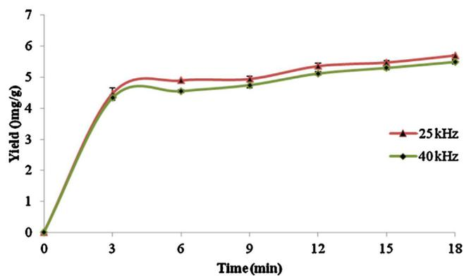
Fig. 6. Effect of ultrasound frequency on extraction yield of piperine from *Piper longum* (ethanol as solvent, extracting time of 18 min, solid/solvent ratio of 1:10, temperature of 40 °C, ultrasonic power of 175 W).
